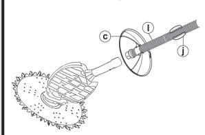
Before attaching the cleaner head, measure the suction flow at the hose the furthest away from the Skimmer box. Keep hose under water and connect the Pool Pulse to the hose using the Quick connector.
