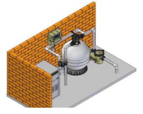
Once the cell is located, connect the black multi-core cable to the cell. The blue wire must be connected to the blue terminal. The cable is designed to come from below the cell. Make sure wing nuts are correctly tightened to ensure good contact.
