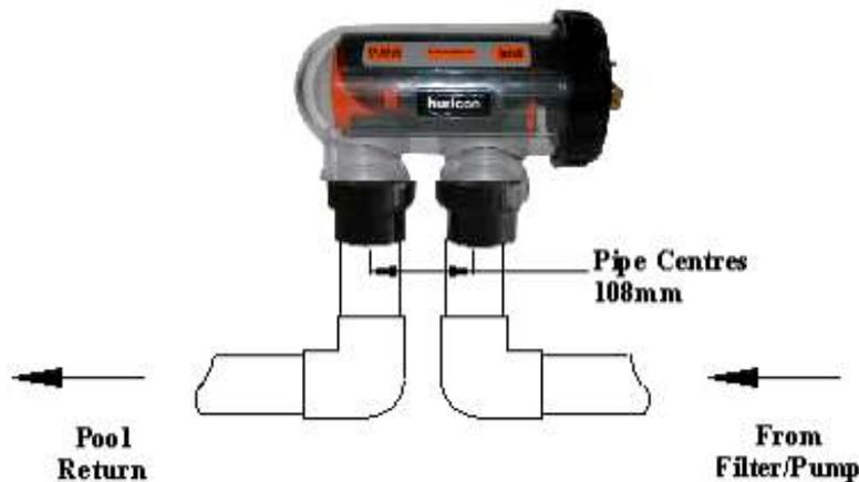
**WARNING:** It is essential that pipe work and equipment do not allow gases generated from the cell to collect and build up.
